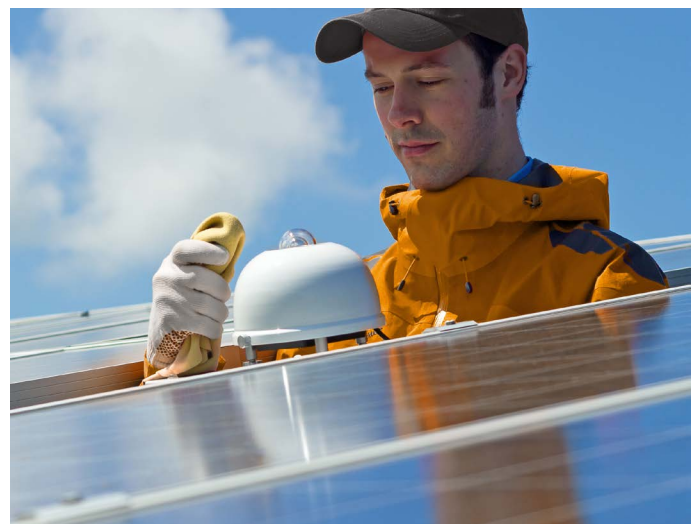
Figure 3 Outdated solution: example of an externally ventilated pyranometer, here in use for PV system performance monitoring.
