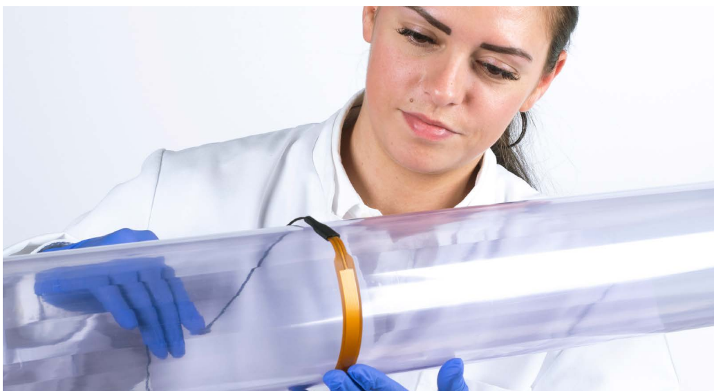
Figure 0.2 Model FHF05-15X85 foil heat flux sensor being installed to measure heat flux on a pipe.
