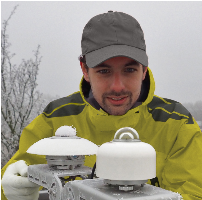
Figure 5 Heating counters frost and dew deposition: clear difference between a heated (right) and non-heated (left) pyranometer.
