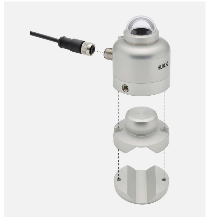
Figure 3 'Exploded view' of SR05. The optional ball leveling and tube mount allow for easy installation. The cable (standard 3 m) features an M12-A connector.
