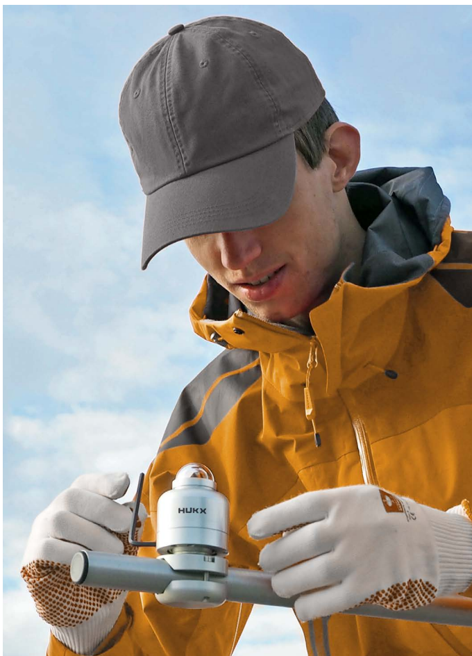
Figure 2 Easy leveling and installation of SR05 with its unique tube mount with ball leveling (optional). SR05 series also offers various industry-standard digital and analog outputs.
