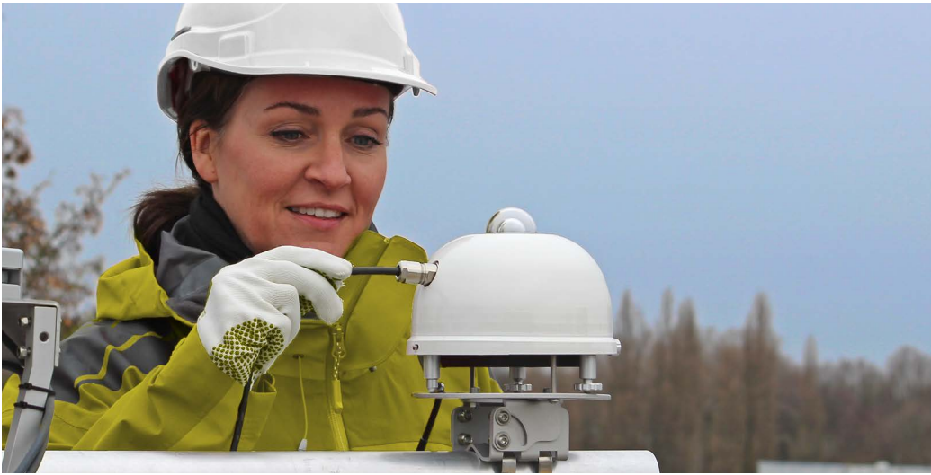
Figure 0.5 VMA01 is a mounting adapter allowing installations on PMF01 of the small footprint VU01 ventilation unit with a suitable Hukx pyranometer, horizontally or tilted.
