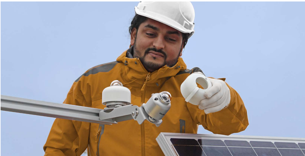
Figure 0.6 PMF02 is uniquely designed for PV system performance monitoring with two pyranometers, one in Plane of Array.
