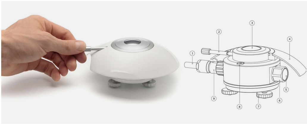
Figure 4.2.1 Installation and removal of IR20's sun screen.
