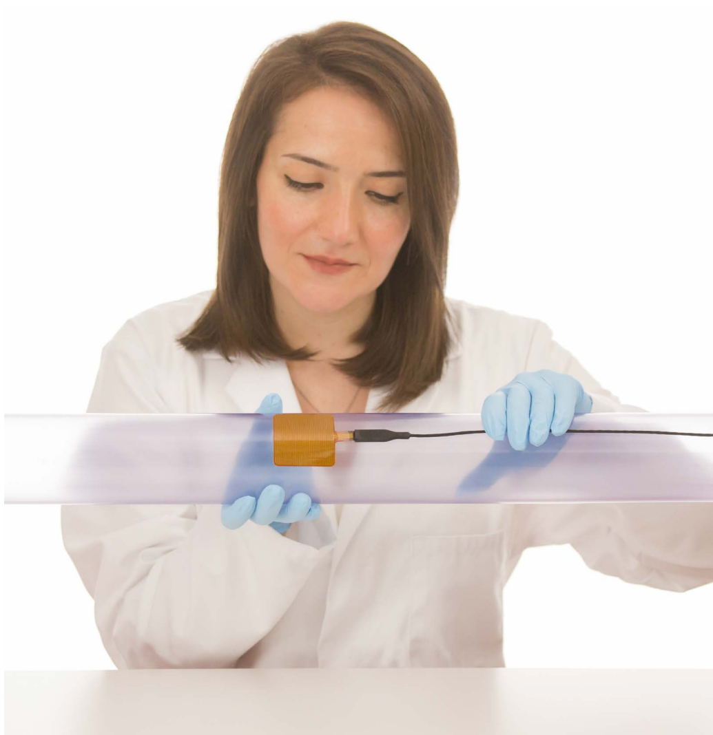
Figure 2 FHF05SC-50X50 being installed to measure heat flux on a curved surface.
