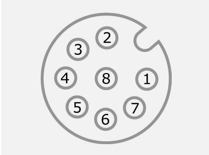
Figure 5.3.1 Connector layout of DR20 / DR15 connector (male), indicating PIN numbers.
