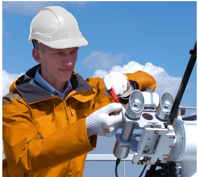
Figure 2 The importance of heating: tracker-mounted operation of heated DR20-A1 and DR15-A1 pyrheliometers being installed with heated SR15-A1 pyranometers. The data availability of non-heated instruments suffers in almost all environments due to morning dew and frost.
