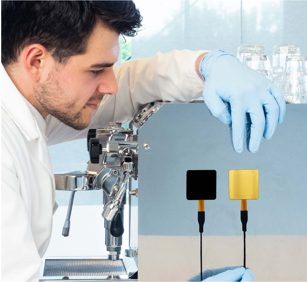
Figure 0.2 Working with BLK – GLD stickers: measuring the radiative and convective heat fluxes on an espresso machine.
