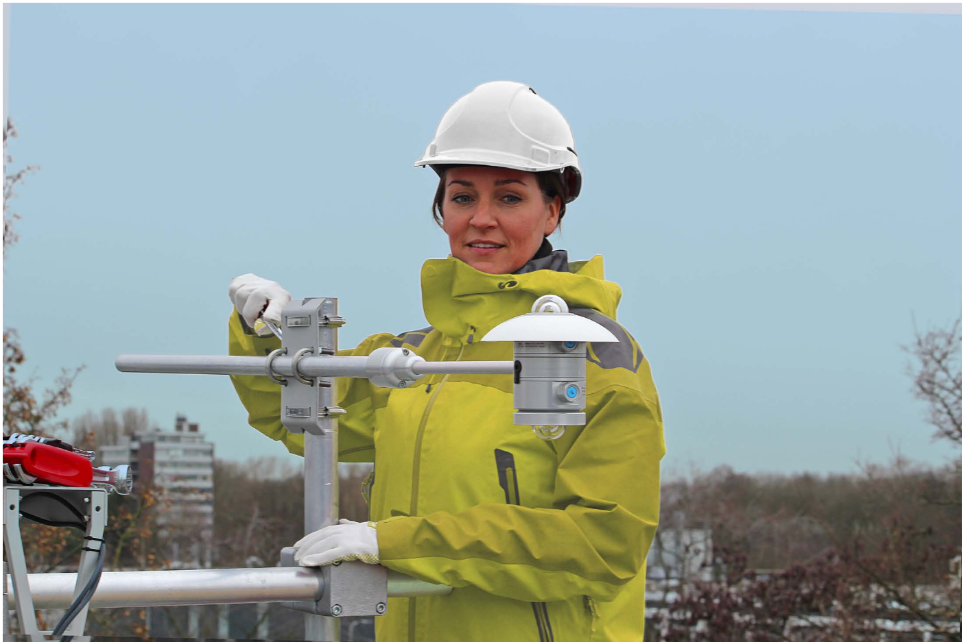
Figure 3.4.3 Installation of an albedometer mounted with AMF02 albedometer mounting fixture and leveled with ALF01 albedometer leveling fixture. The crossarm mounting fixture, connecting the cross arm to a vertical mast is CMF01.
