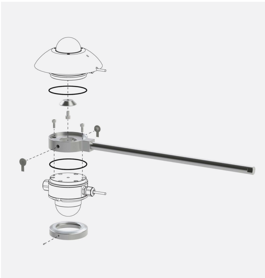
Figure 3.2.1 AMF02 with 2 x SR11, mounting and fixation steps 1 to 8.
