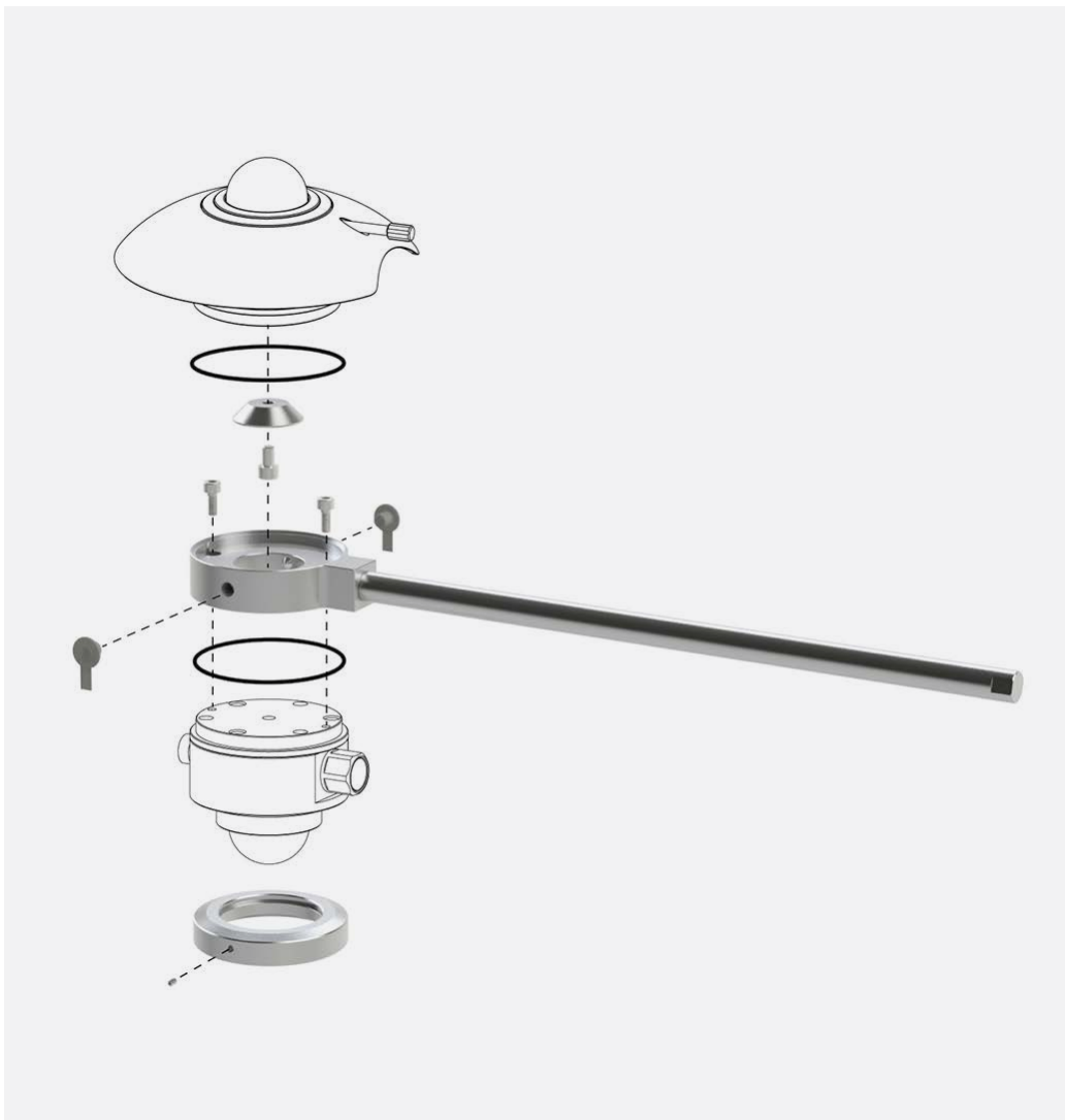
Figure 3.2.2 AMF02 with 2 x SR20(-D2), mounting and fixation steps 1 to 8.
