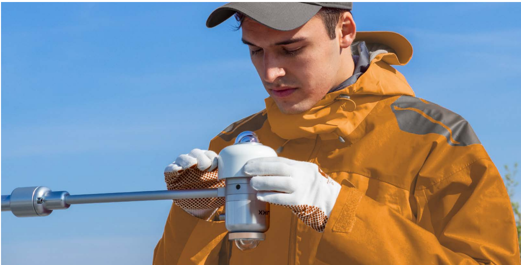
Figure 0.4 Installation with AMF03, two SR30-M2-D1 pyranometers and ALF01 leveling fixture.
