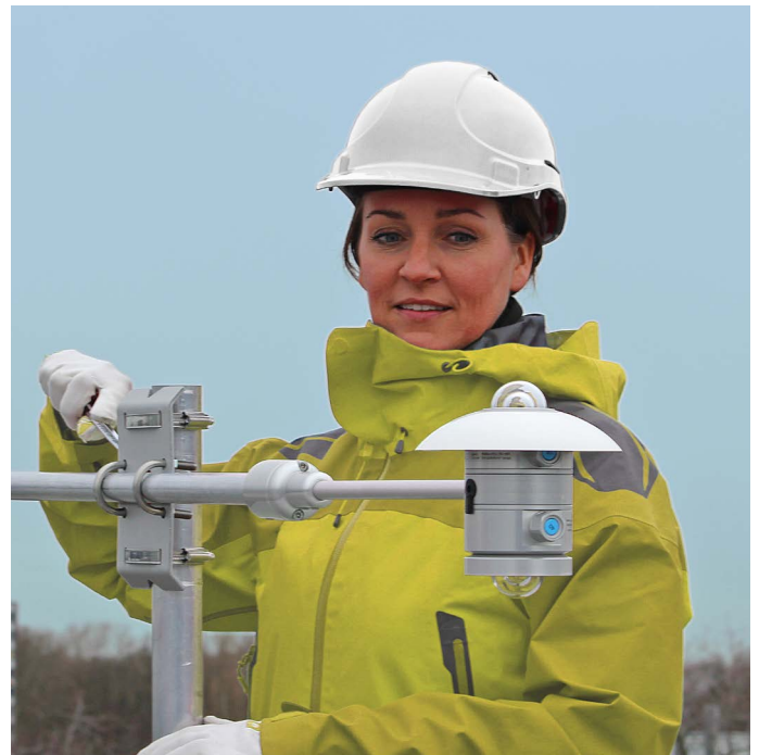
Figure 6 Installation of AMF02 albedometer mounting kit and two SR20 pyranometers, mounted with ALF01 leveling fixture on a crossarm with crossarm bracket CMF01.
