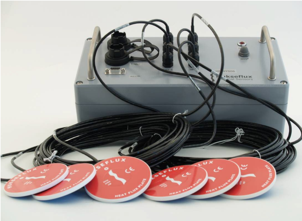
Figure 1 HFPSYS06 consists of MCU Measurement and Control Unit and six heat flux sensors. Readout is performed by connecting temporarily to a PC (not included). Software for readout (Loggernet) is included.
